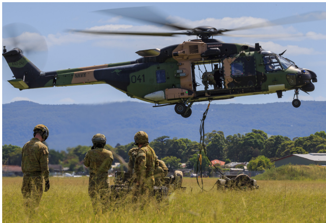
Australian Army soldiers from 176th Air Dispatch Squadron conduct an external lift training activity with a Royal Australian Navy MRH-90 Taipan helicopter. Credit: CoA / Jack Brock
