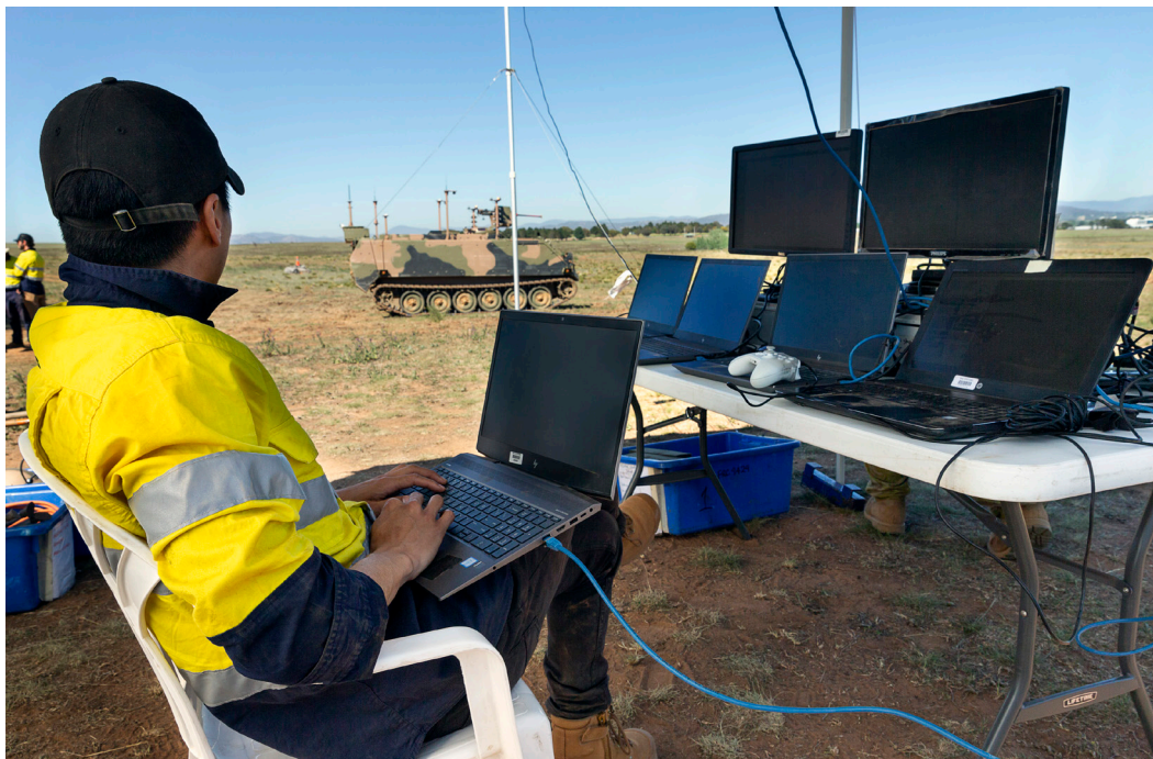
A technician from BAE Systems Australia remotely inputs controls to an autonomous M113 AS4 optionally crewed combat vehicle (OCCV) at the Majura Training Area, Canberra. Credit: CoA / Tristan Kennedy
