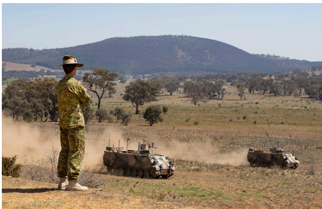
Australian Army officer Brigadier Ian Langford, DSC and Bars, watches on as two autonomous M113 AS4 optionally crewed combat vehicle (OCCV) assault an enemy position at the Majura Training Area, Canberra. Credit: CoA / Tristan Kennedy
