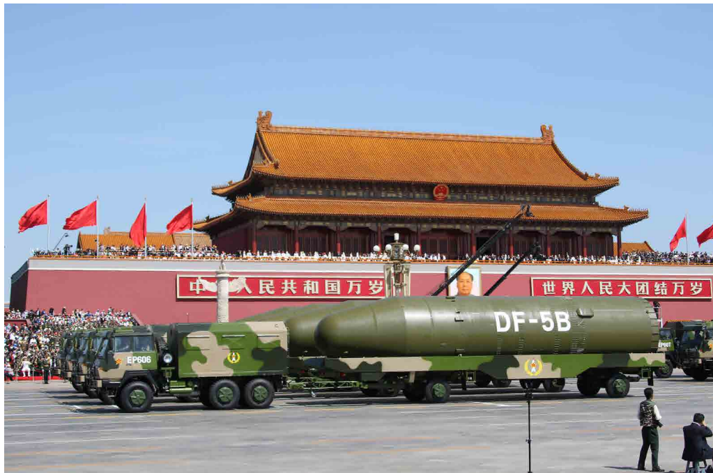
The DF-5 series of ICBMs are liquid-fuelled, and they are launched from underground silos. Pictured here is the warhead and upper stage of a DF-5B. (Gordon Arthur)
