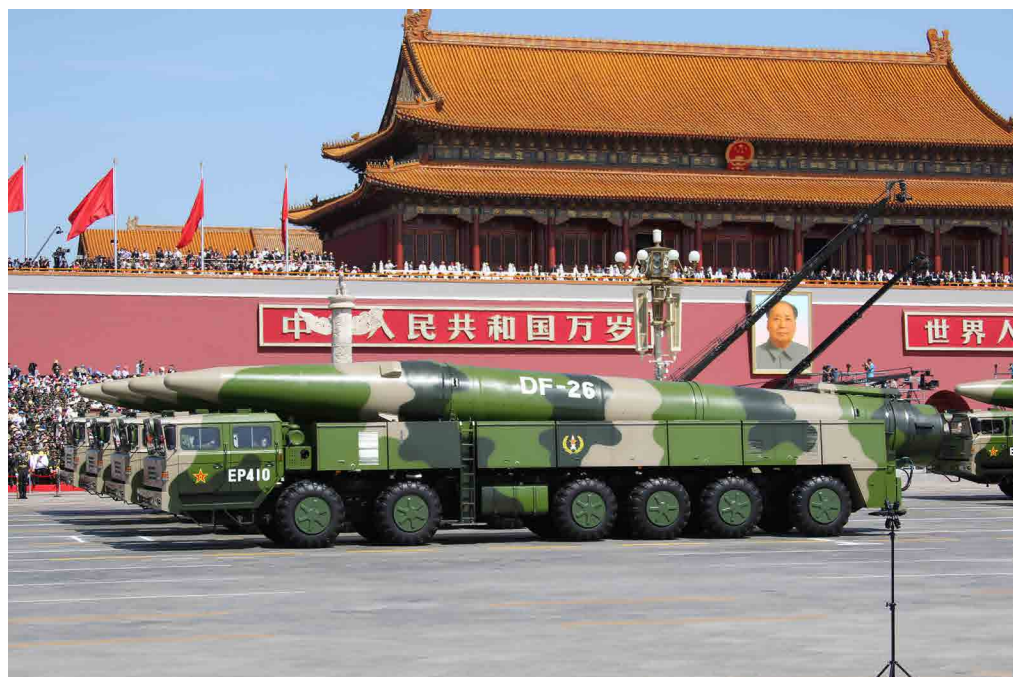
The DF-26 is one of China’s most important ballistic missiles. This intermediate-range missile can carry either a conventional or nuclear warhead. (Gordon Arthur)
