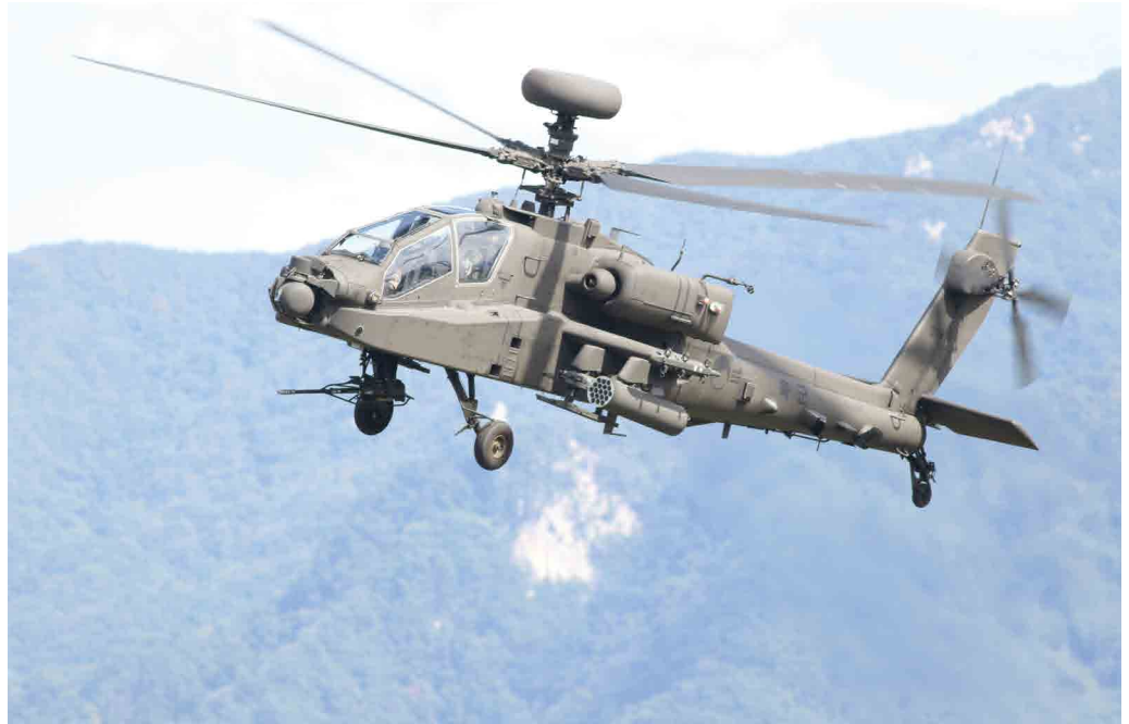
AH-64E Apache attack helicopters can be fitted with either the Longbow radar (as here) or an MUM-T antenna, but not both at the same time. (Gordon Arthur)
