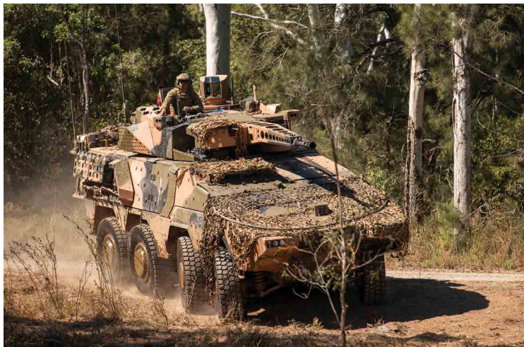
This is a Boxer with the Lance turret mounting Rheinmetall's MK30-2 ABM cannon. The Lance turret is fitted to 133 of Australia's 211 Boxer vehicles. (ADF)
