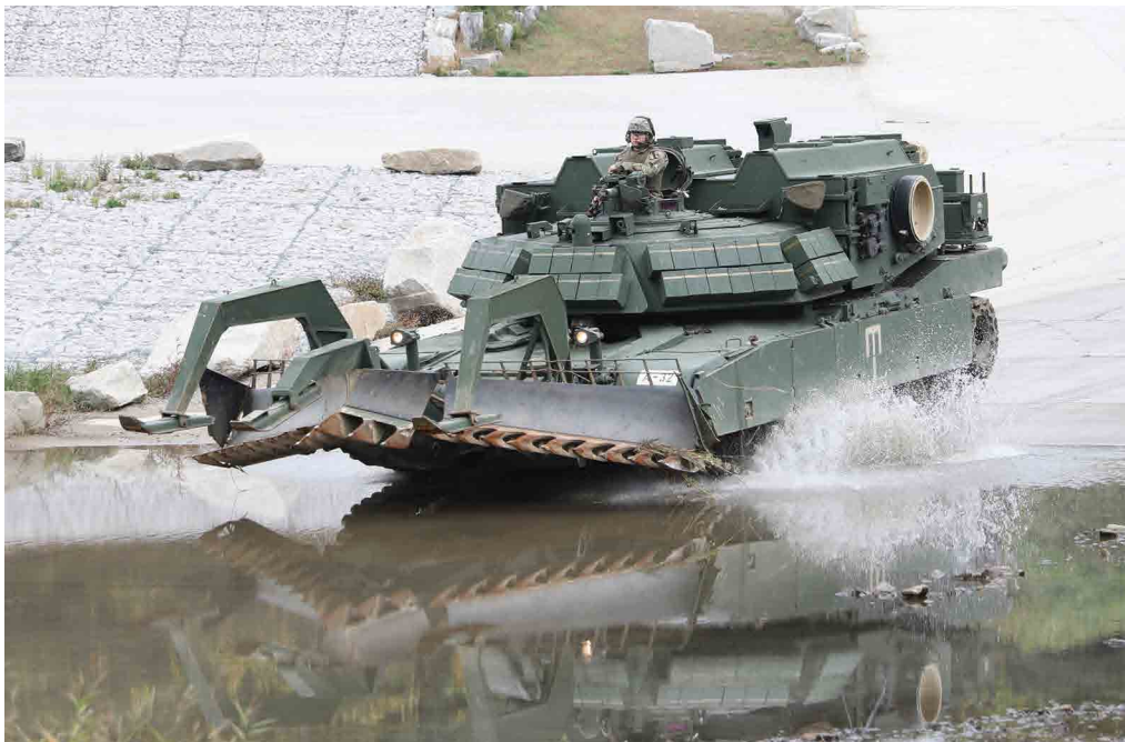
This M1150 Assault Breacher Vehicle of the US Army was photographed in South Korea. Australia will receive 29 examples of the ABV. (Gordon Arthur)
