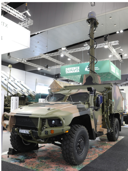
This two-door Hawkei vehicle carries Raytheon's AN/AAS-52 Multispectral Targeting System, seen here extended on its mast. (Gordon Arthur)
